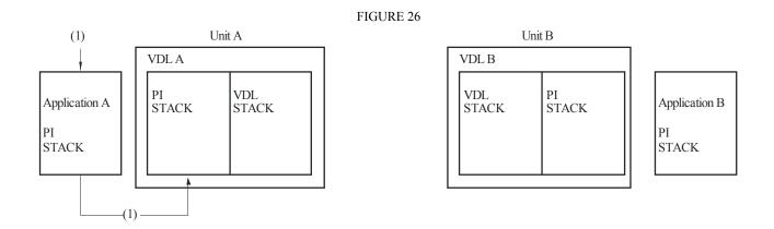
Step 1: Application A delivers 4 addressed messages addressed to B with sequence numbers 0, 1, 2 and 3 via PI.
