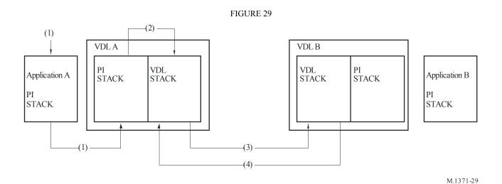
Step 4: DL B returns VDL-ACK messages with sequence numbers 0 and 3 to VOL A.
