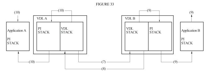
Step 8: VDL B successfully receives Message 2 and returns a VDL-ACK with sequence number 2. Step 9: VDL B delivers ABM (addressed binary message) message with sequence number 2 to Application B.
