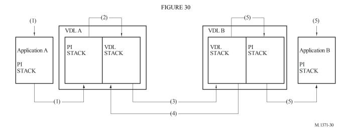
Step 5: VDL B delivers addressed messages with sequence numbers 0 and 3 to Application B.
