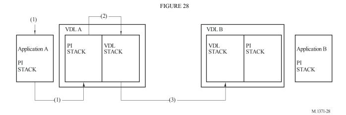
Step 3: VDL A transmits the messages to VDL B, which only receives messages with sequence numbers 0 and 3.
