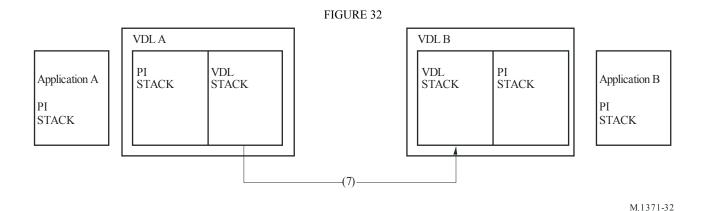
Step 7: VDL A times out on sequence numbers 1 and 2 and retransmits the addressed messages to VDL B.
