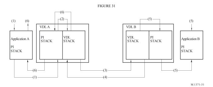
Step 6: VDL A returns PI-ACK (OK) to Application A with sequence numbers 0 and 3.
