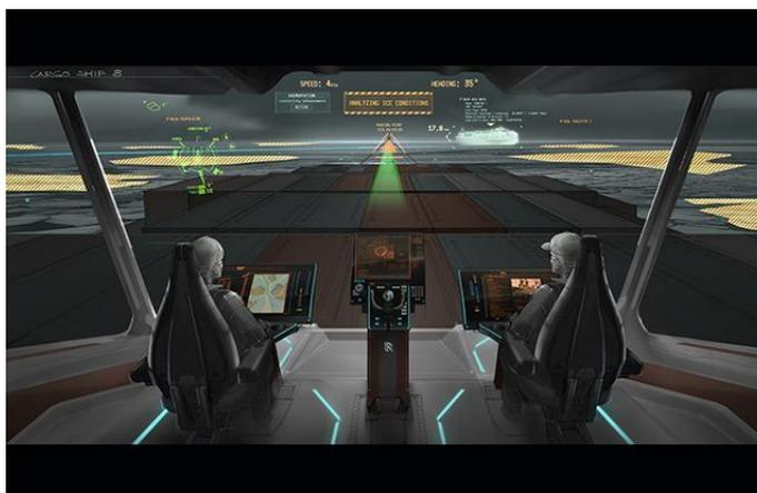
In this image you can see a version of augmented reality on the screen – displaying the ship's route, speed and other characteristics as well as the characteristics and routes of other ships.
