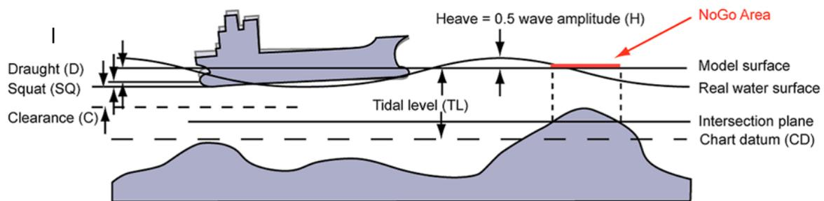
$$\text{Depth of the intersection plane} = \text{TL}(t) - \text{D}(t) - \text{SQ}(v) - \text{C} - \text{H}(t)$$
